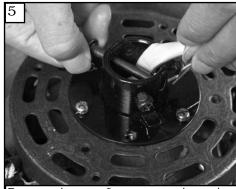
Remove keeper from cross pin and then cross pin from yoke. Replace keeper on cross pin and save.
